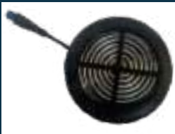
2. The visible part (around the electrode ring) is cleaned with a cleaning brush to remove all the impurities deposited.
