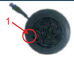
1. Hold the generator in one hand and pick up the clamp position (arrow 1) with the finger of the other hand. The cover can be removed.
